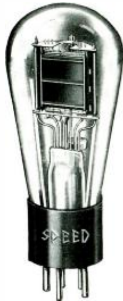
247 New power amplifier Pentode, for use in the output stage of AC receivers.
